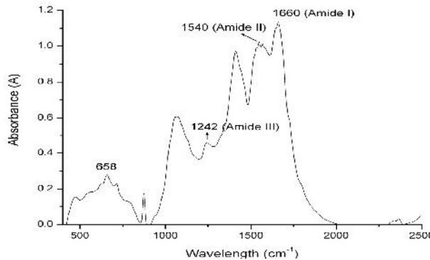
**FIGURE 3.** FT-IR spectra of sericin from *A. assamensis* in the spectral range of  $400\text{--}4000\text{cm}^{-1}$
