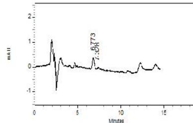
Fig: 5 HPLC profile of Aflatoxin in soil
