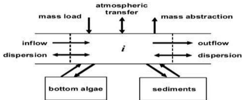
FIGURE 3 Mass balance in a reach segment i. Source: (Pelletier and Chapra, 2005)
