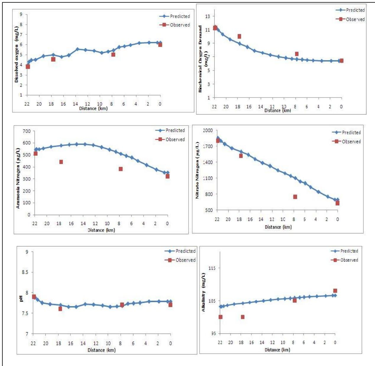
**FIGURE 5** Model calibration results for the water quality parameters in Karanja River using Pre-monsoon data
