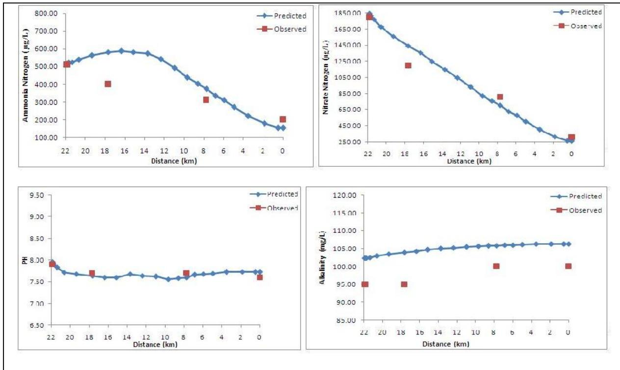
FIGURE 6. Model validation results for the water quality parameters in Karanja River using Post- monsoon data
