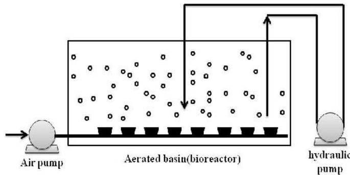
**FIGURE 2.** Schematic representation of the bioreactor
