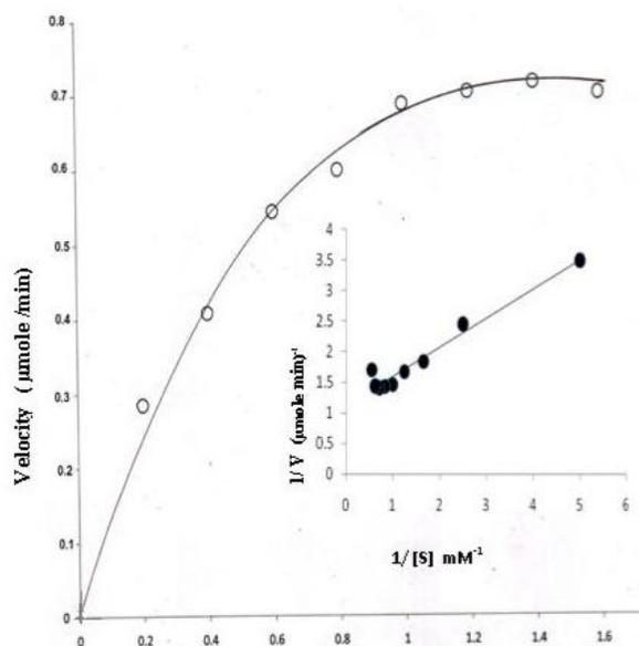
**FIGURE 6.0** Michaelis-Menten curve (a) and double reciprocal plot (b) for the laccase of *A. biennis* MTCC-1176 using DMP as the variable substrate. In (a) and (b) 1 mL reaction solution contained 0.0-2.0 mM DMP, 50 μL of the enzyme stock (8 μM) in sodium malonate buffer pH 4.5 at 25 °C.
