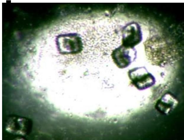
**FIGURE 8.0** Enzyme crystals in 0.05 molar potassium phosphate and 20% polyethylene glycol 8000 in 20 μL droplet containing enzyme 0.5 mg/mL.
