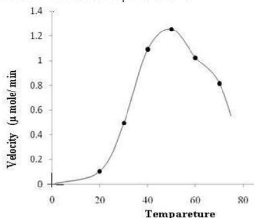
**FIGURE 7.0 (b)** Determination of temperature optimum of the purified enzyme. In this case 1 mL reaction solution contained 1.0 mM DMP in 100 mM sodium malonate buffer pH 4.5 with varying temperature from 20 to 100 °C. 50 μL of the enzyme stock (8 μM) was used.
