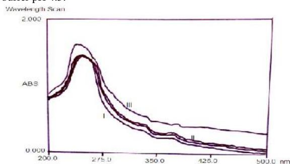
**(b)** UV/Visible spectrum of biotransformation of methyl benzene to benzaldehyde using purified yellow laccase in the absence of mediator molecule (details in the text). Spectrum I is just after mixing the reagents and the closed two spectra marked as II are after 10 min and 20 min of mixing the reagents. Spectrum III is after 24 hrs of mixing the reagents
