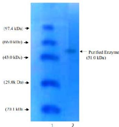
**FIGURE 3.0** SDS-PAGE of the purified laccase. Lane 1 contains molecular weight markers and lane 2 contains 20 $\mu\text{g}$  of the purified enzyme.
