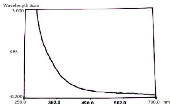
**FIGURE 4.0 (a)** UV/Visible spectrum of the purified enzyme (8.04  $\mu$ molar) with reference to 10 mM sod. acetate/ acetic acid buffer pH 4.5
