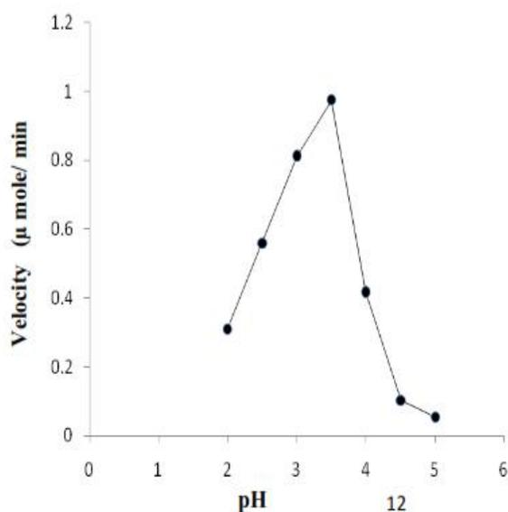
**FIGURE 7.0 (a)** Determination of pH optimum of the purified enzyme. In this case 1 mL reaction solution contained 1.0 mM DMP in 100 mM sodium malonate buffer with varying pH from 2.0 to 5.0 and temperature was fixed at 25 °C. 50 μL of the enzyme stock (8 μM) was used.
