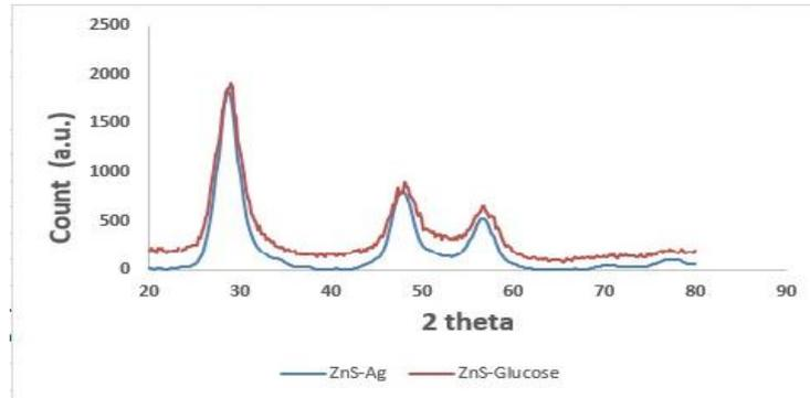
FIGURE 1: XRD of ZnS, ZnS-Ag nanoparticles with 2 theta
