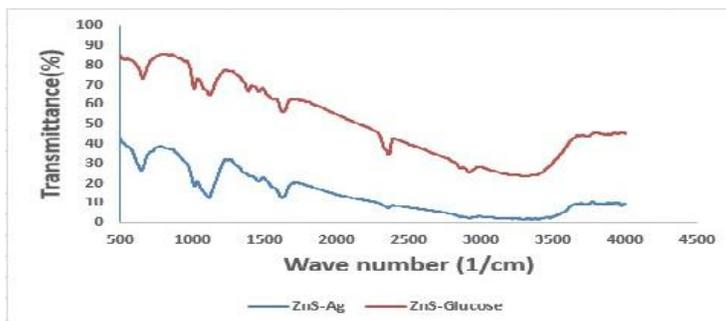
**FIGURE 3:** FTIR spectra of ZnS-Ag nanoparticles
