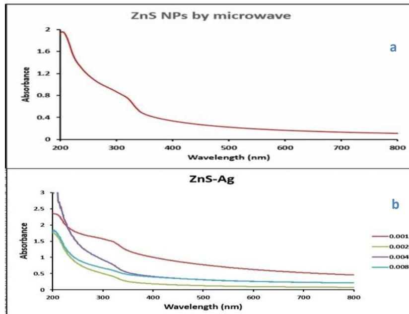
FIGURE 2: UV-Vis Absorption spectrum of (a: ZnS and b: ZnS-Ag) nanoparticles
