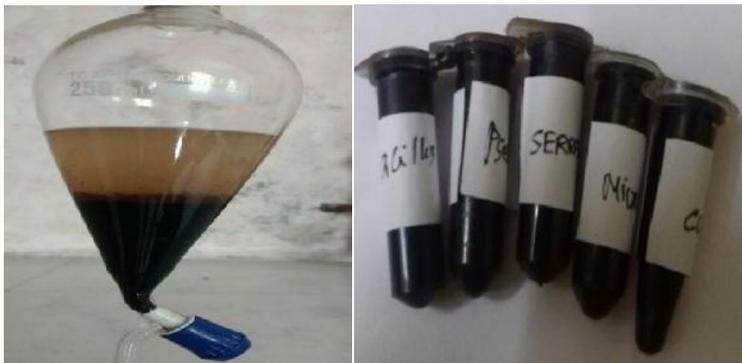
Figure 3 a) Extraction of residual oil Figure 3 b) Extracted residual oil
