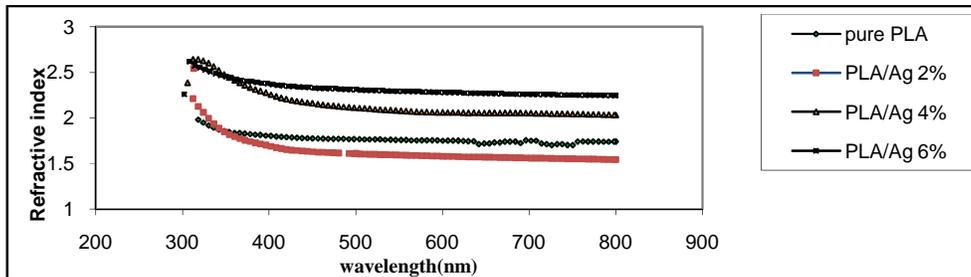
FIGURE 4: The variation of refractive index (n) versus wavelength for PLA and PLA/Ag nanocomposites
