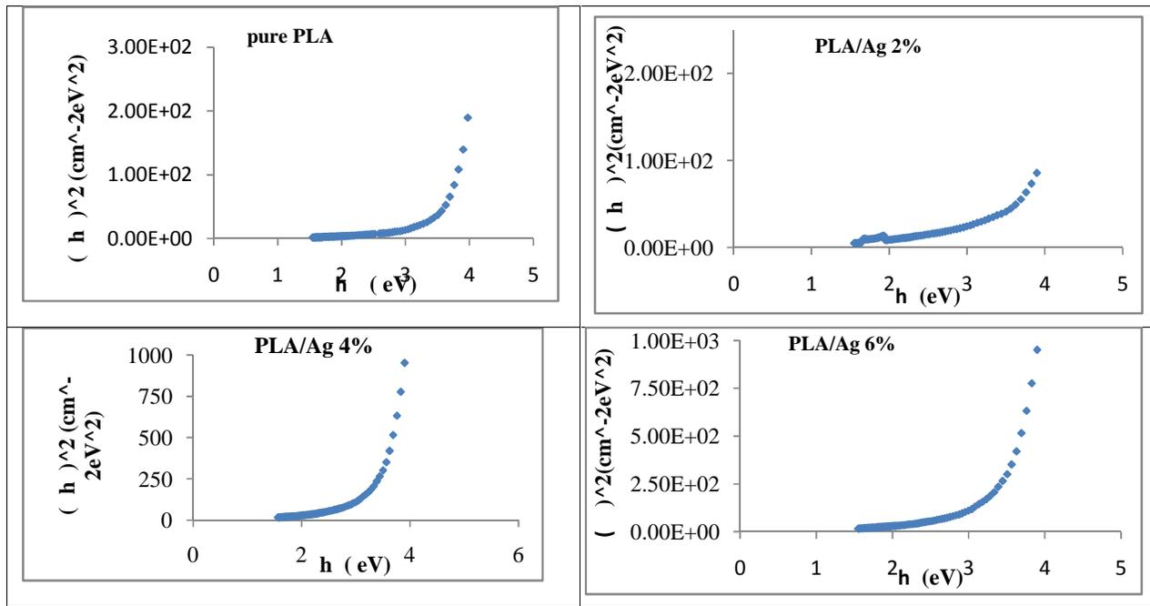
FIGURE 3: The variation of  $(h)^2$  versus  $(h)$  for pure PLA and PLA/Ag nanocomposites
