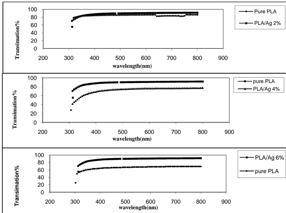
**FIGURE 2:** Transmittance as function to wavelength for PLA, PLA/Ag nanocomposites
