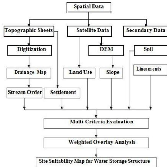
**FIGURE 2:** Flowchart for Identifying Suitable Location of Water Storage Structure
