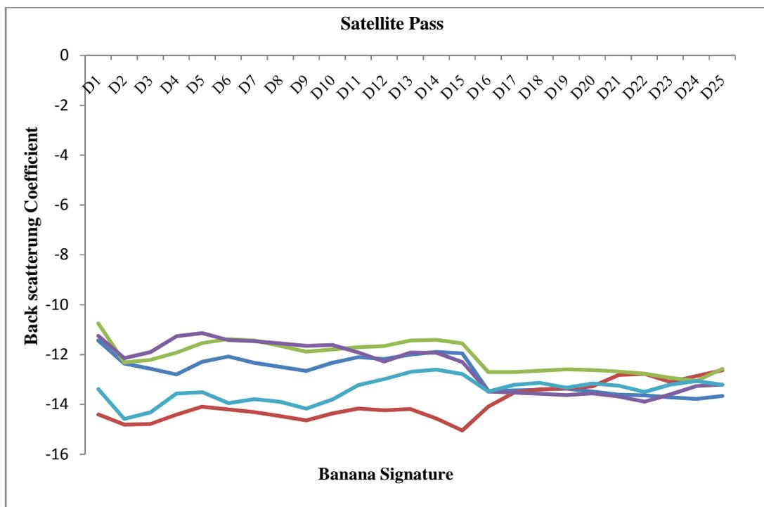
FIGURE 2 .Temporal back scattering signature of banana crop in VH polarization at different GT points
