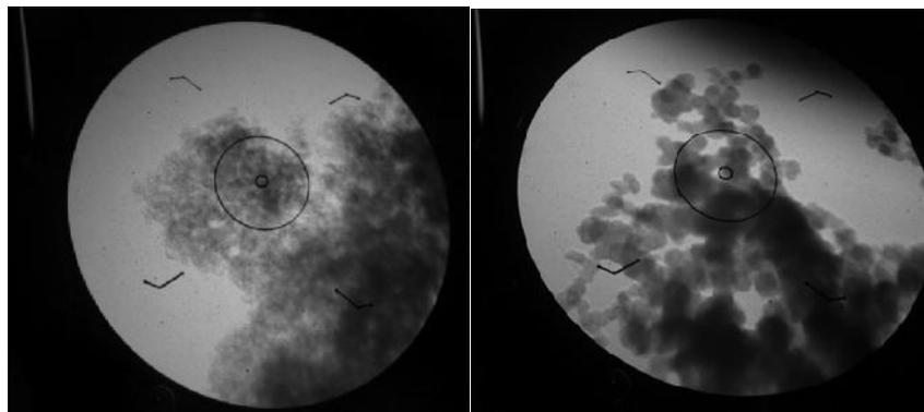
**FIGURE 6:** TEM images of AuNPs at concentration (a) 1 mM (b) 5 mM
