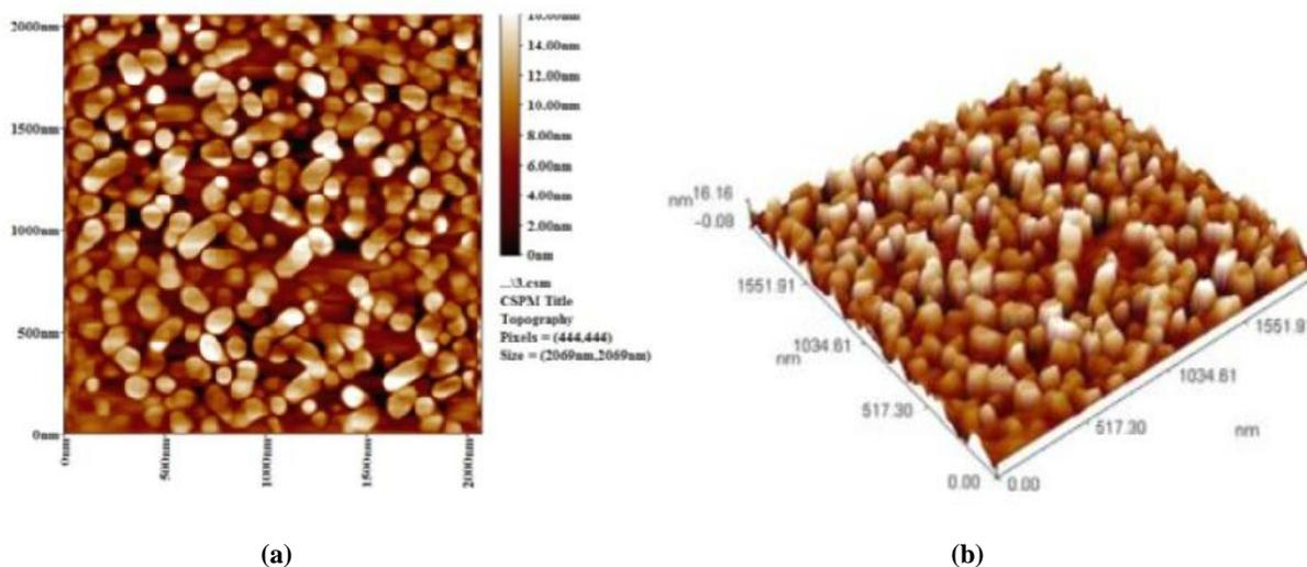
**FIGURE 7:** explain image of AFM of AuNps for concentration 1 mM, (a) two dimensions, (b) three dimensions, (c) histogram of distribution of grain size.
