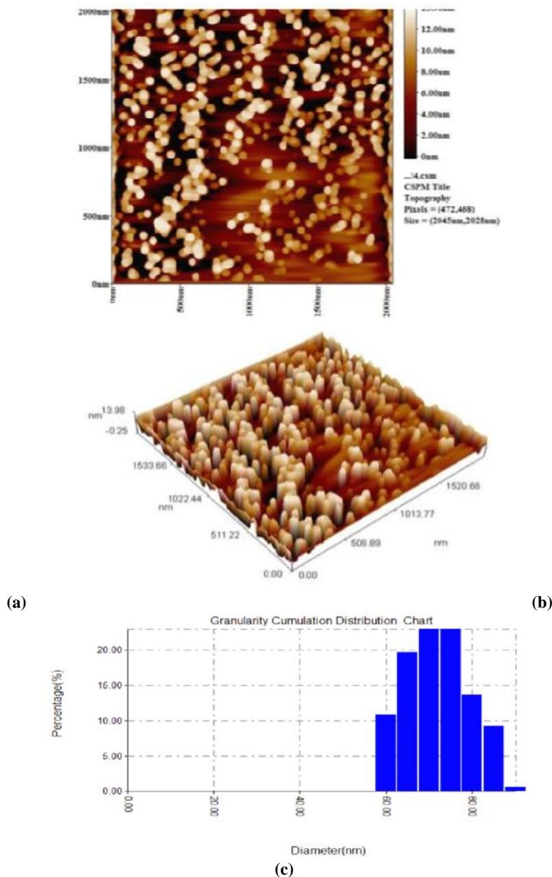
**FIGURE 8:** explain image of AFM of AuNps for concentration 5mM (a) two dimensions, (b) three dimensions, (c) histogram of distribution of grain size.
