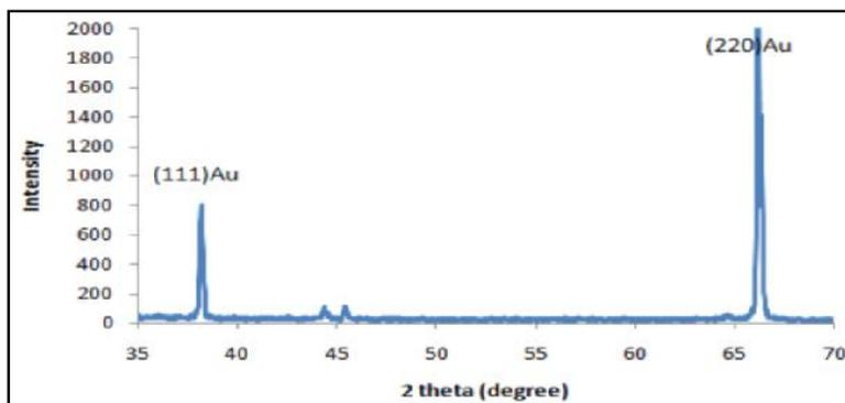
FIGURE 5: XRD pattern of AuNPs at 5 mM.
