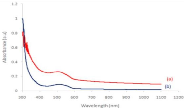
**FIGURE 9:** UV-Visible absorbance spectra of AuNPs for HAuCl<sub>4</sub>.3H<sub>2</sub>O with aqueous extract of sumac at concentration, (a) 5 mM and (b) 1 mM.
