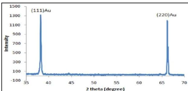
FIGURE 4: XRD pattern of AuNPs at 1mM.
