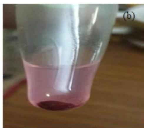
FIGURE 3: produced samples of AuNPs explain the change in color from orange to ruby red at (a) 5mM (b) 1mM.
