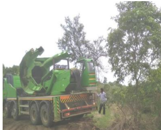
b. Tree Transplanter machine and transplantable tree
