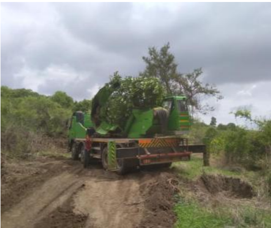
c. Tree Transplanter machine with uprooted tree
