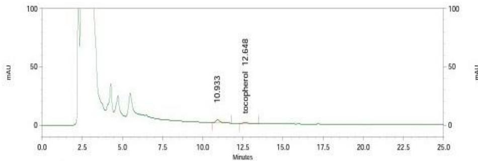
**FIGURE 3:** Chromatogram of tocopherol of mechanically extracted linseed oil
