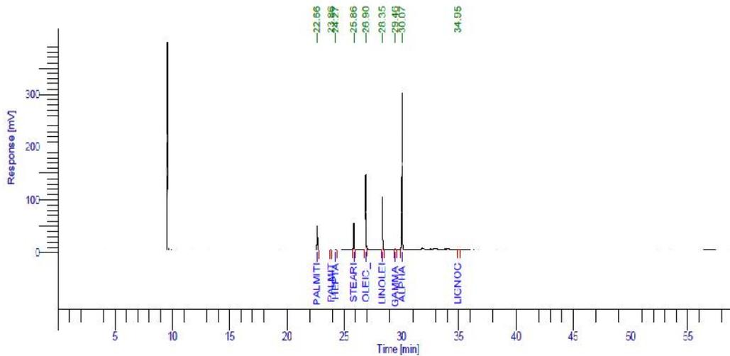
**FIGURE 2:** Fatty acids chromatogram of solvent extracted linseed oil
