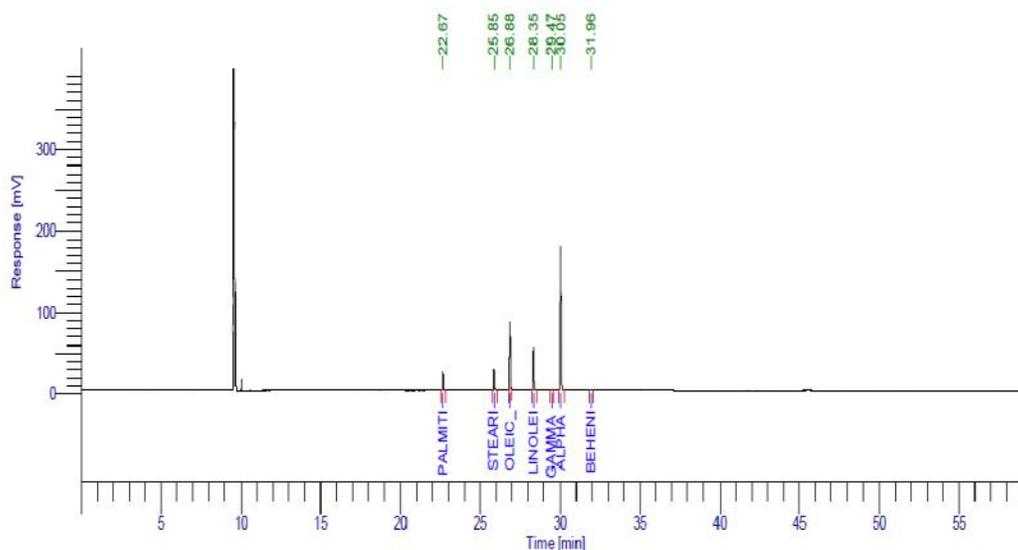
**FIGURE 1:** Fatty acids chromatogram of mechanically extracted linseed oil
