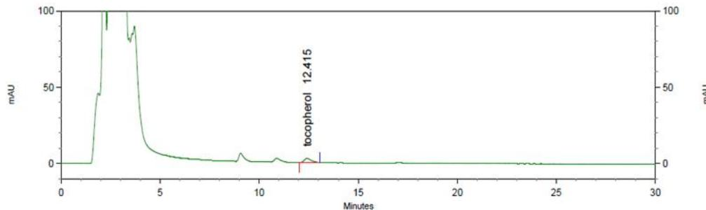
**FIGURE 4:** Chromatogram of tocopherol of solvent extracted linseed oil
