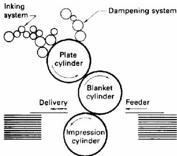
Fig 1. Conventional Offset printing Machine
