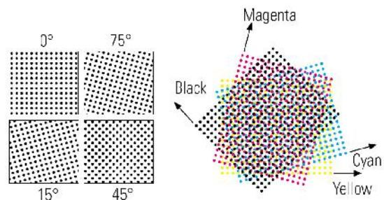
Fig 3. Color angles used in offset printing
