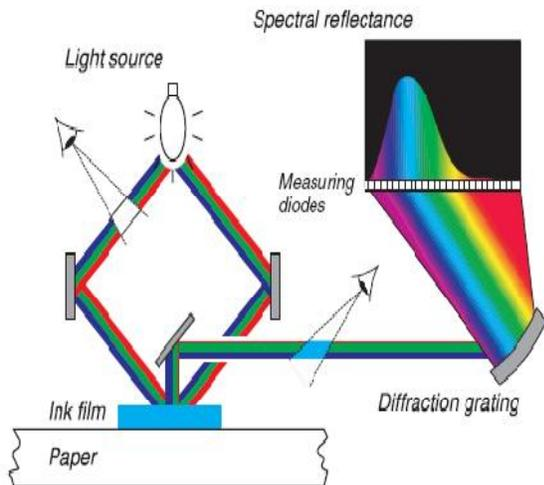
Fig 4. Principle of Spectrophotometer
