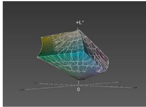
The 3d visual gamut comparison between visual gamut and gamut printed by sequence of KCMY, showing min. Delta E and Max. gamut volume.
