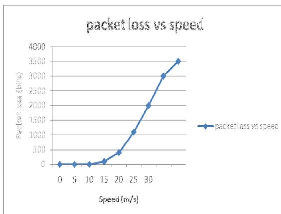
Fig 5- Impact of node Speed On Packet Loss
