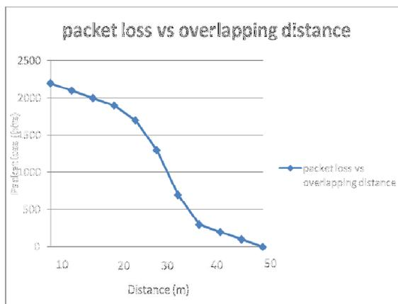
Fig 7- Impact of overlapping distance on packet loss
