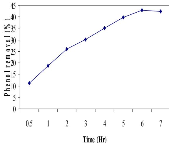
**Fig. 2.** Kinetics for phenol removal; Initial phenol concentration (10 mg/L); Adsorbent dose (200 g/L), Solution pH 6.
