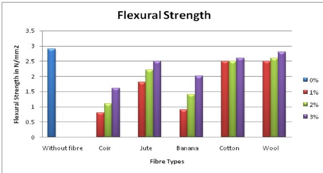
**Figure 3 Effects of fibre type and proportion on flexural strength**
