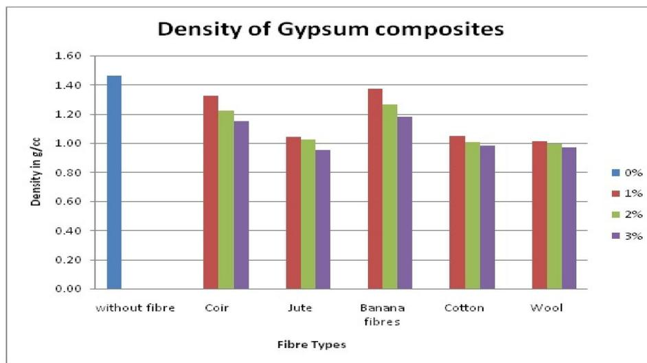
**Figure 6 Effect of fibre reinforcement on density of gypsum composites**
