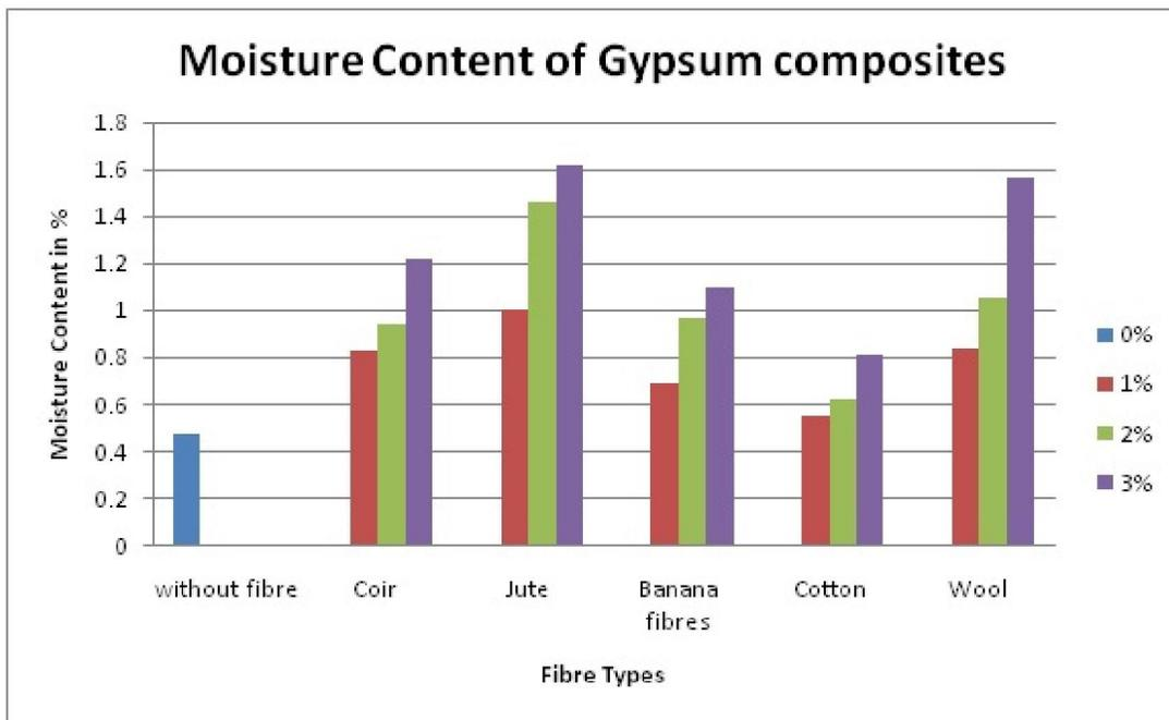
**Figure 5 Effects of fibre reinforcement on moisture content of gypsum composites**
