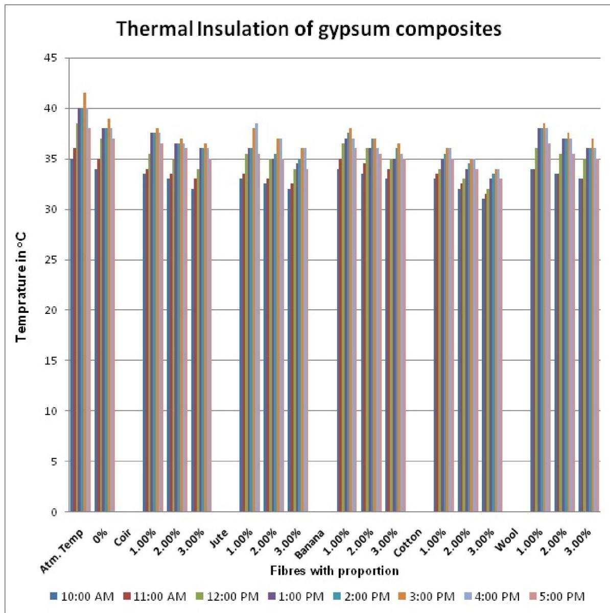
Figure 4 Effects of fibre reinforcement on thermal insulation
