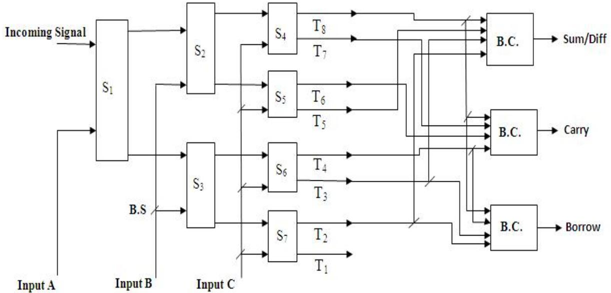
Fig.2. Schematic diagram of full adder-subtractor using SOA based MZI switches (BC: Beam Combiner, BS: Beam Splitter).
