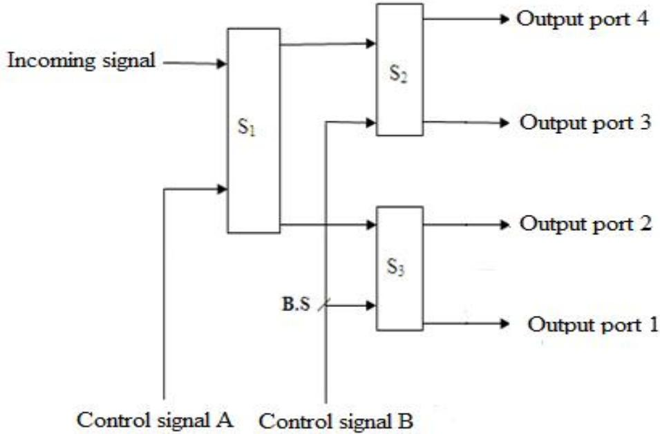
Fig.5.Schematic diagram of demultiplexer.
