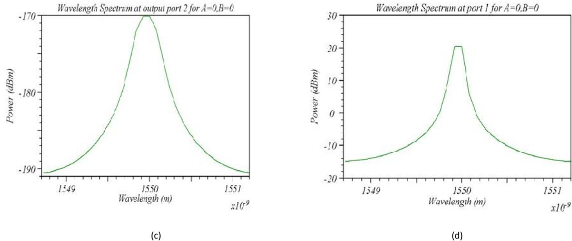
Fig.6. Demultiplexer output at different ports for  $A=B=0$ . (a) Output port 4 (b) Output port 3 (c) Output port 2 (d) Output port 1
