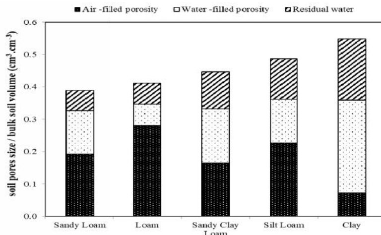
FIGURE 2. Air and water distribution in three soil sample, Air-filled pore volume (pores >9.03 \times 10^{-04} cm) and water-filled pore volume (pores <9.03 \times 10^{-04} cm, water + residual water)
