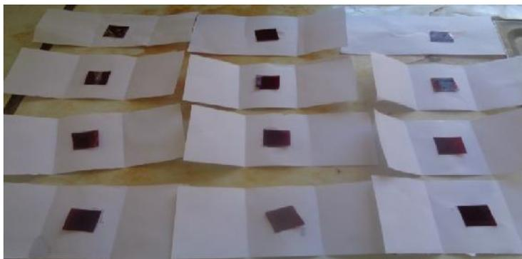
**FIGURE 1:** Drying LR-115 detectors after chemical etching
