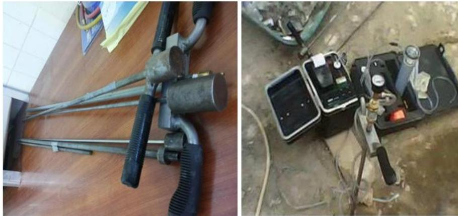
**FIGURE 7:** The RAD-7 soil-gas setup, including the electronic radon monitor
