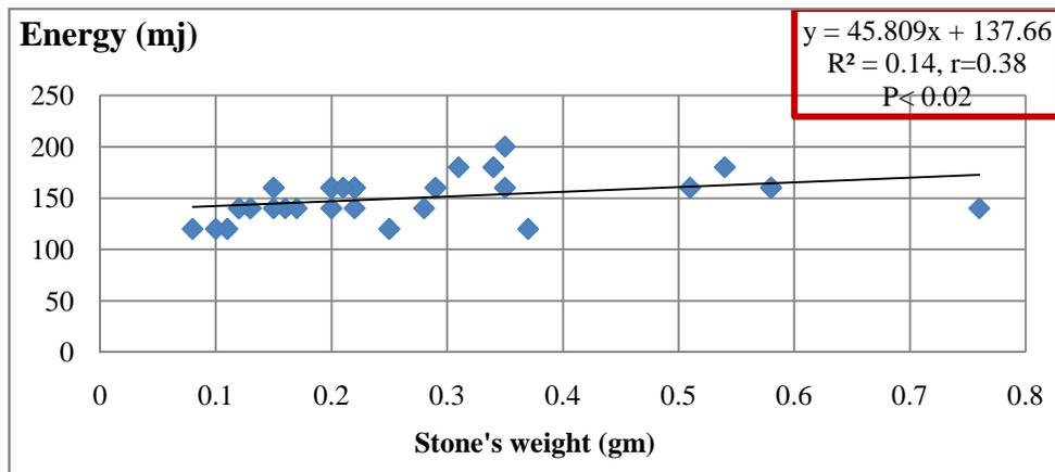
In the current study, as the frequency of the Nd: YAG laser was doubled to 1064nm, the results showed a direct and significant correlation between the weight of the uric acid calculi and the laser's energy which were required to break the these stones ( $P<0.02$ )
