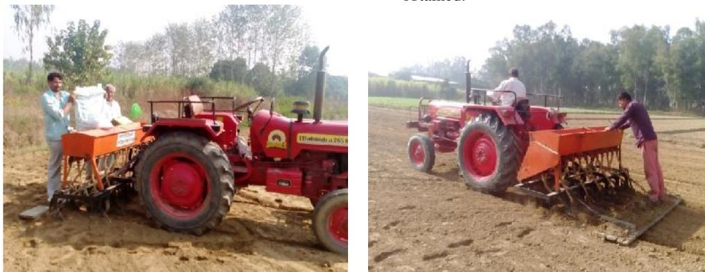
FIGURE 1:- Tractor operated seed cum fertilizer drill
