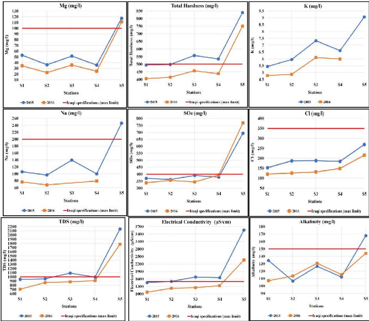
**FIGURE 3:** (pH, Temperature, DO, PO<sub>4</sub><sup>-3</sup>, NO<sub>3</sub>, Ca<sup>+2</sup>, Mg<sup>+2</sup>, T.H, K<sup>+1</sup>, Na<sup>+1</sup>, SO<sub>4</sub>, Cl, TDS, EC, and Alkalinity) variations in the Euphrates River for the years 2015 and 2016.
