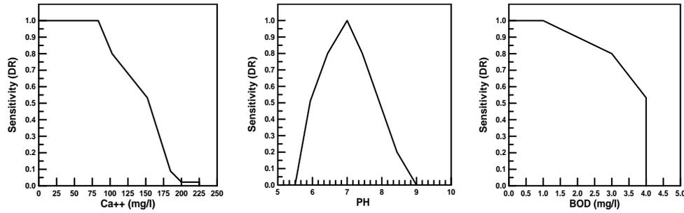
FIGURE 2: Sensitivity functions curves according to Bhargava WQI method for drinking purpose.
