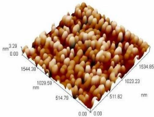
**FIGURE 5:** The AFM images of AgNPs prepared with the volume ratio of extract to AgNO<sub>3</sub> (2:10) ml
