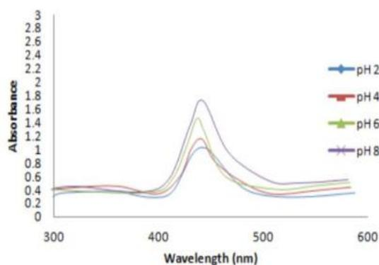
FIGURE 10: The UV spectrum of AgNPs prepared at different PH
