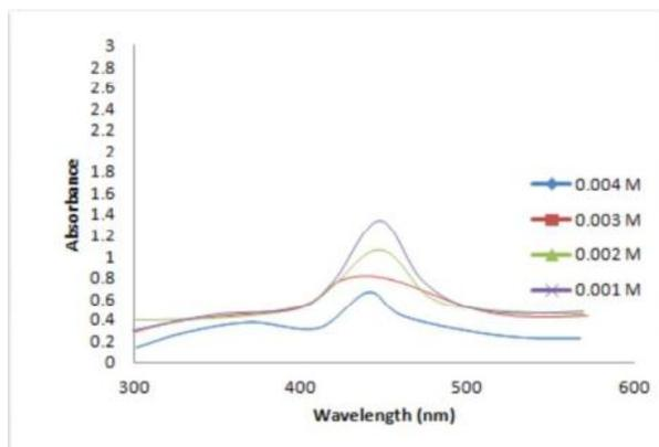
FIGURE 8: The UV spectrum of AgNPs prepared with different conc. of silver ion
