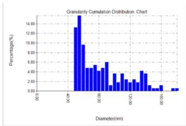
**FIGURE 7:** The scanning probe microscopy shows the cumulation distribution of granules prepared using 6:10 volume ratio of extract to AgNO<sub>3</sub>.
