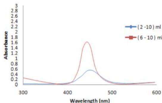
FIGURE 9: The UV spectrum of AgNPs prepared with different volume ratio of extract to AgNO<sub>3</sub>
