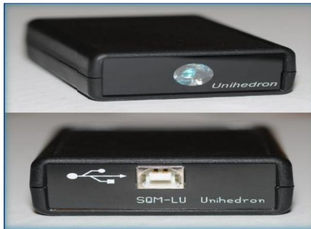
FIGURE 5: Sky Quality Meter; model LU (front and back of unit)<sup>[14]</sup>
