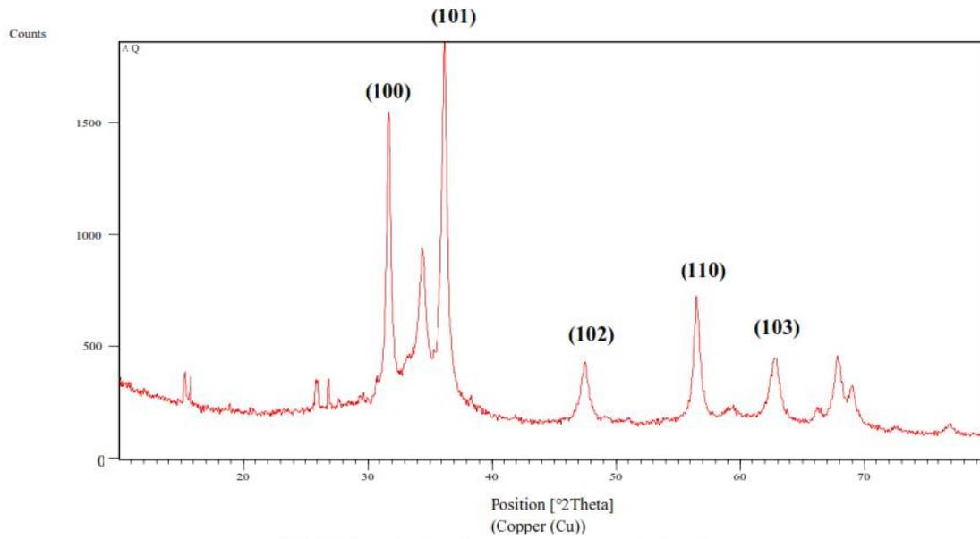
FIGURE 5: X-Ray Diffractogram of AZnO-NPs
