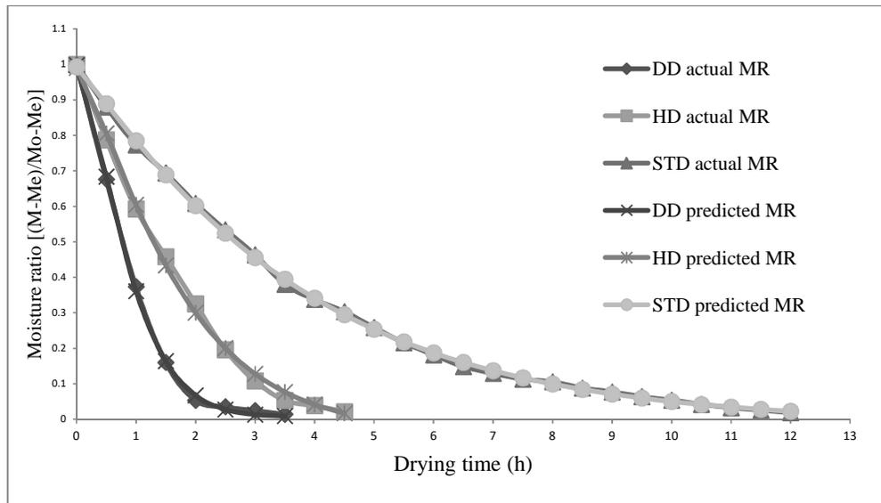
**FIGURE 2:** Experimental and midilli-kucuk model predicted moisture ratio for different drying methods (Abbreviation: STD, solar tunnel drying; HD, hot air drying; and DD dehumidified drying)
