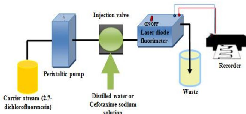
FIGURE 2: Manifold that used for determination of cefotaxime sodium based on fluorescence quenching
