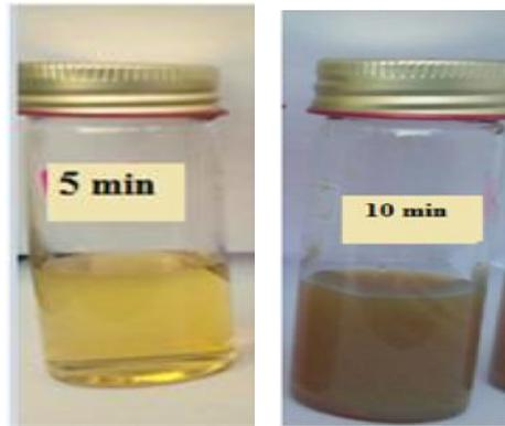
FIGURE 1: prepared silver Nanoparticles by a hot chemical reduction method with 5 and 10 min reduction periods
