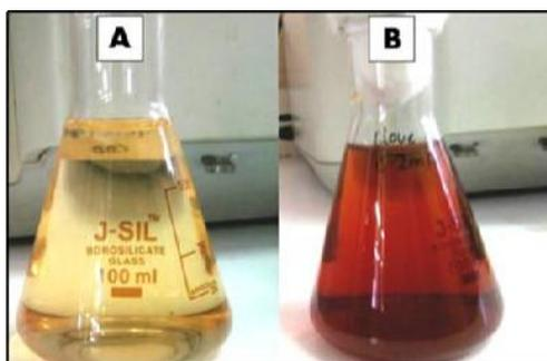
**FIGURE 1:** Biological synthesis of silver nanoparticles. A: Initial colour of *S. aromaticum* extract with AgNO<sub>3</sub> (0 minutes). B: After 24hrs incubation
