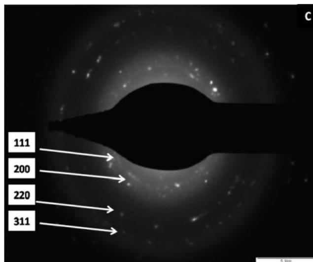
**FIGURE 3A.** Transmission electron microscope of silver nanoparticles (Scale bar is 100 nm), B. Particle size distribution of biologically synthesized nanoparticles and C. Selected area electron diffraction (SAED) of silver nanoparticles (Scale bar is 5 1/nm).
